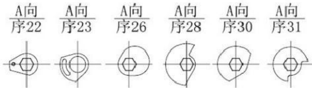
Position diagram of the brake sector of the operating shaft
